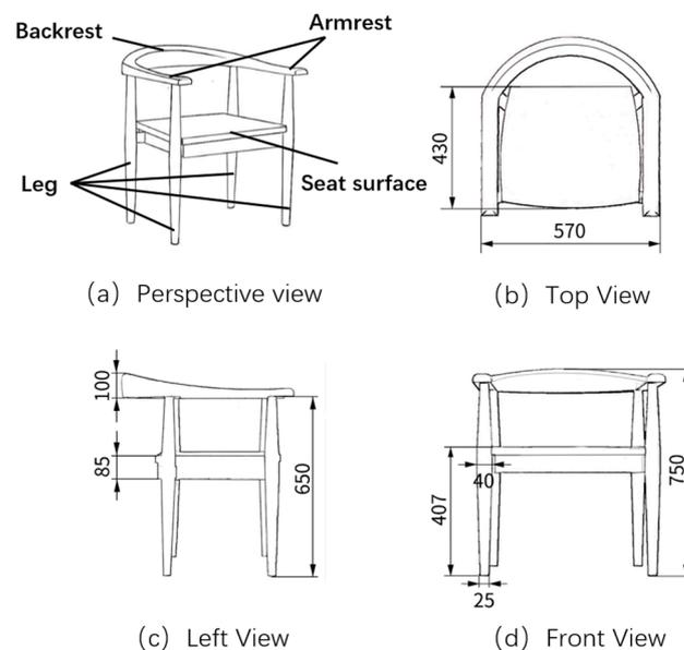
**Figure 2.** Perspective view and three views of a traditional armchair.
