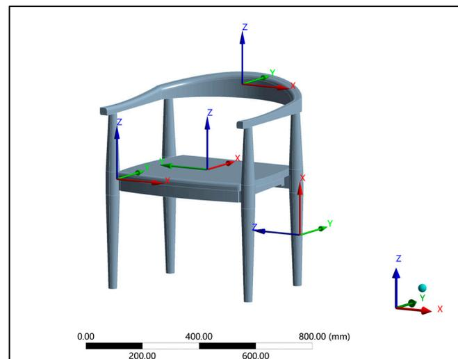
**Figure 3.** Material orientation of each component of the chair.
