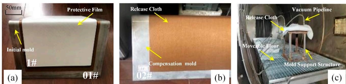
**Figure 9.** Autoclave process of curing experiment: (a) initial mold and uncured composite components; (b) compensated manufacturing die obtained in this paper; (c) field diagram of curing test.
