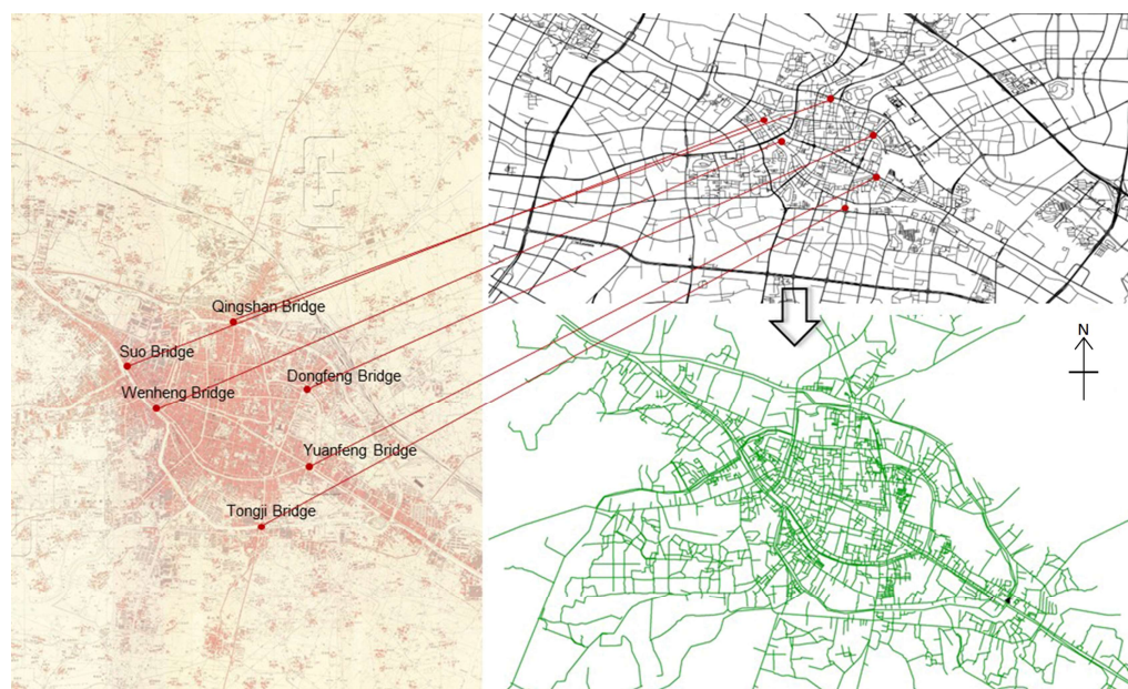
Figure 4. The diagram illustrates the method of translating historical maps. The left image depicts a historical map from the 1970s, while the upper right image displays a street map with a coordinate system from 2021. The lower right image shows the road map from the 1970s after translation using ArcGIS 10.5.
