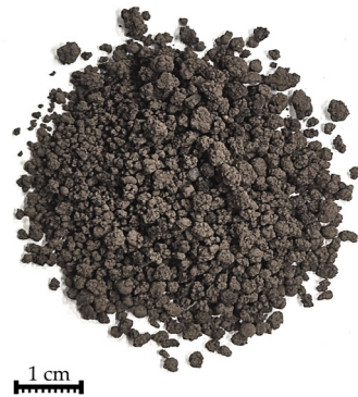
Figure 7. Microgranules made of steel mill dust, slag former, carbon carrier, and water in an Eirich mixer type EL1.
