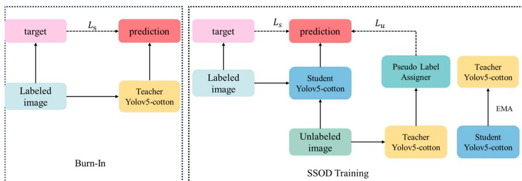
Figure 5. Efficient YOLOv5-cotton foreign fiber detection model training process.
