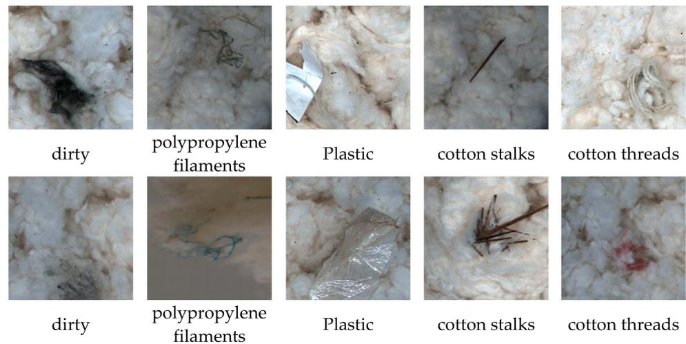
**Figure 2.** Data samples (the foreign fiber types are not divided and the same label, “large fiber”, is used).
