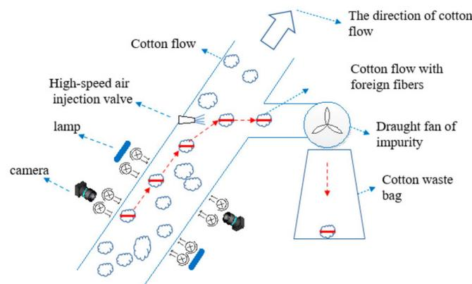
**Figure 1.** Foreign Fiber Splitting Machine.
