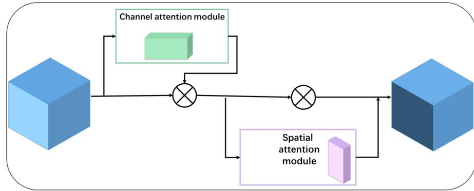
**Figure 6.** CBAM module: the input feature maps are successively weighted by the channel and spatial attention modules to obtain the output feature maps of CBAM.
