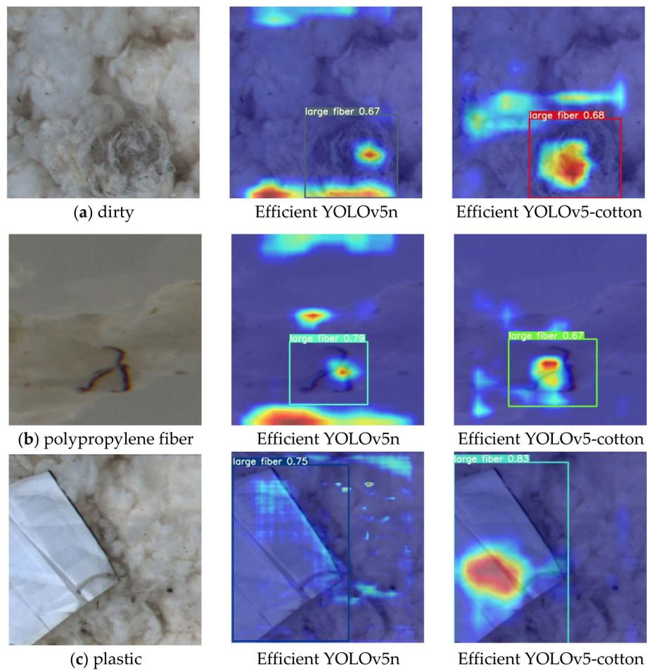
Figure 11. The heat map of Efficient YOLOv5-cotton vs. Efficient YOLOv5n, where the red color represents the current thermal maximum region.
