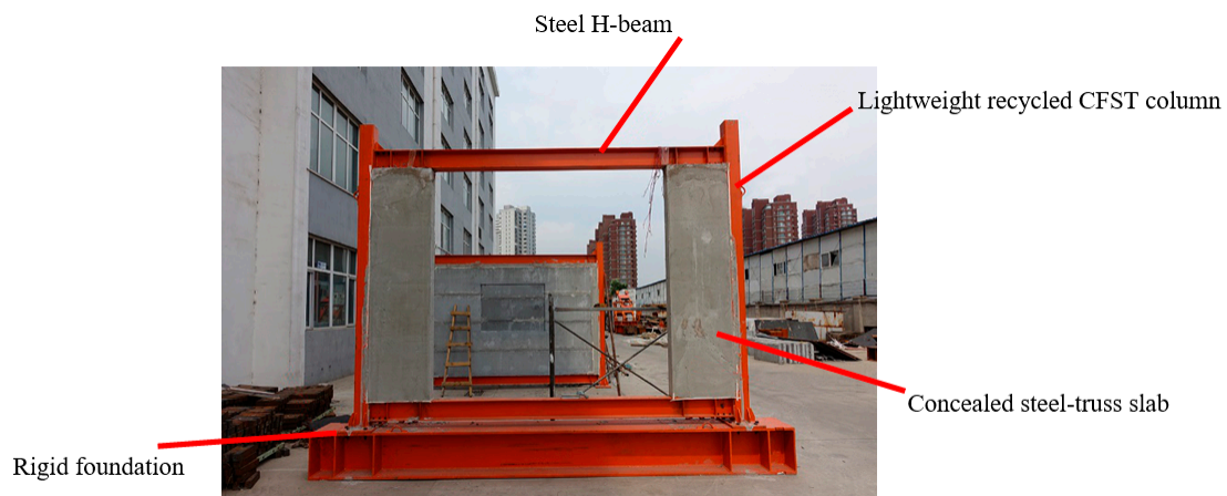
Figure 4. Concealed steel-truss panel.
