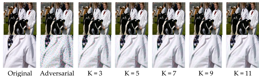
Figure 5. The adversarial examples are obtained by applying various median filtering kernels to process the adversarial perturbations, where K represents the size of the filter kernel.
