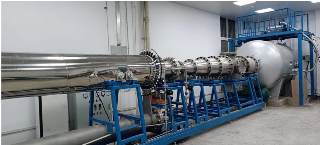
**Figure 1.** HUST's  $\Phi 0.5$  m Mach 6 hypersonic Ludwig wind tunnel.
