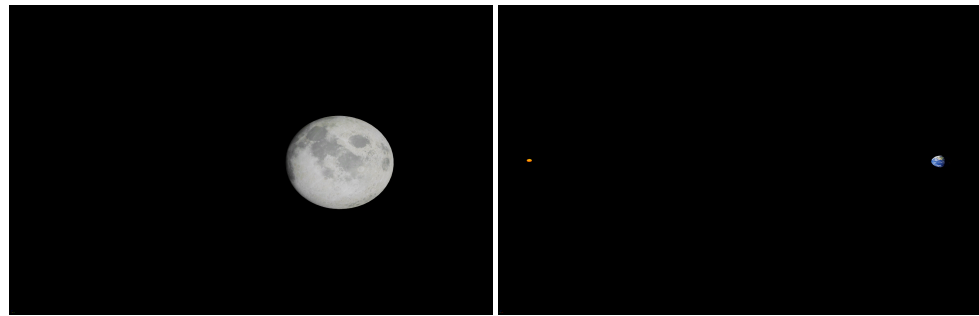
Figure 14. The ESTCube-LuNa real-time 3D (RT3D) navigation concept in Unreal Engine 5 with textures from the Solar System Scope [61]. The image on the left shows the Moon; on the right, the Sun and the Earth, as imaged by two out of five 120° FoV cameras. By imaging three celestial objects, triangulation can be used to determine the ESTCube-LuNa position in lunar orbit, as described in Section 5.5.2.
