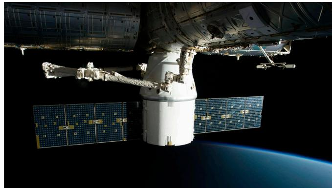
**Figure 1.** The solar panel of a SpaceX spacecraft.
