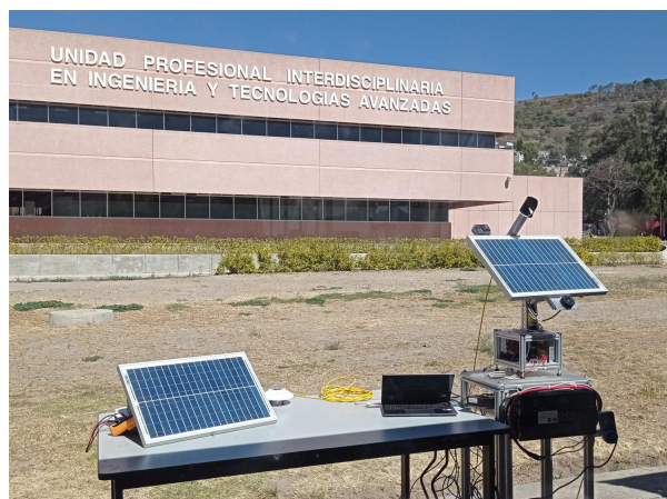
Figure 6. Fixed SC and ST used for performance test for ESC.
