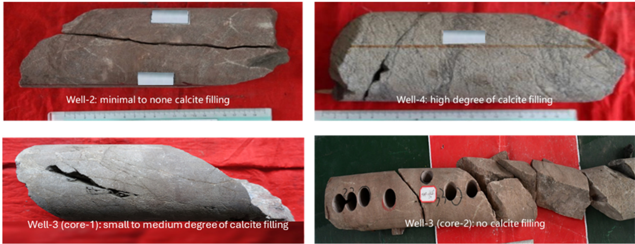
Figure 12. Core data observations of calcite filling across different wells in the reservoir.
