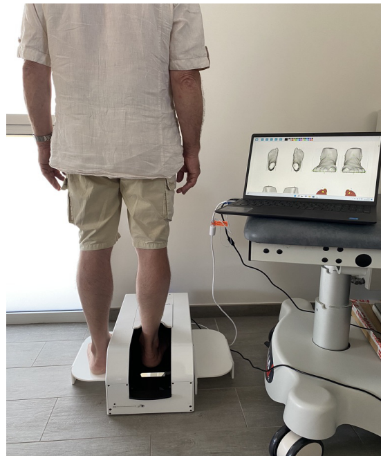
Figure 3. Subjects were positioned standing on both feet: one foot in the scanner, and the other foot on a footrest at the same height (courtesy of Beldame J et al., Assessment of the Efficiency of Measuring Foot and Ankle Edema with a 3D Portable Scanner. Bioengineering , 2023).
