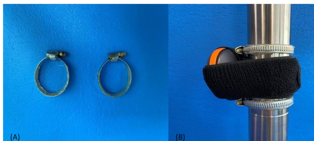
Figure 2. (A) Silicone coated clamps and (B) pole mounting method.
