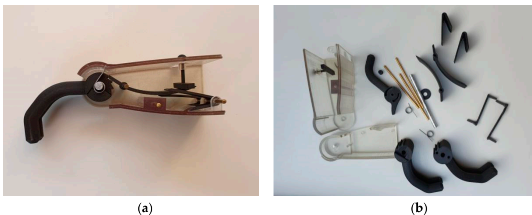
Figure 4. Third 3D-printed polymer replica of the first “Iron Hand” of Götz von Berlichingen with an opening mechanism by a torsion spring. (a) In this photograph, the first finger block, the new thumb lever mechanism, and the lateral chassis cover are removed to see the torsion spring; (b) view of all components after disassembling the hand.
