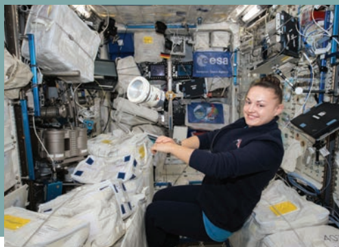
View of Russian cosmonaut Elena Serova as she performs the RJR Augmented Microbial Sampling investigation by taking air samples with Microbial Air Sampler.
