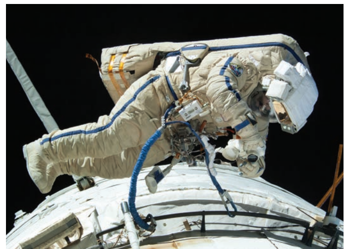
Russian cosmonaut Alexander Misurkin, attired in a Russian Orlan spacesuit (blue stripes), participates in a session of extravehicular activity (EVA) to continue outfitting the International Space Station.
