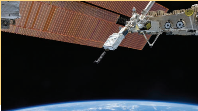
NanoRacks CubeSat Deployer.
