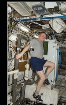
NASA astronaut Mike Fincke uses Cycle Ergometer with Vibration Isolation System (CEVIS).
