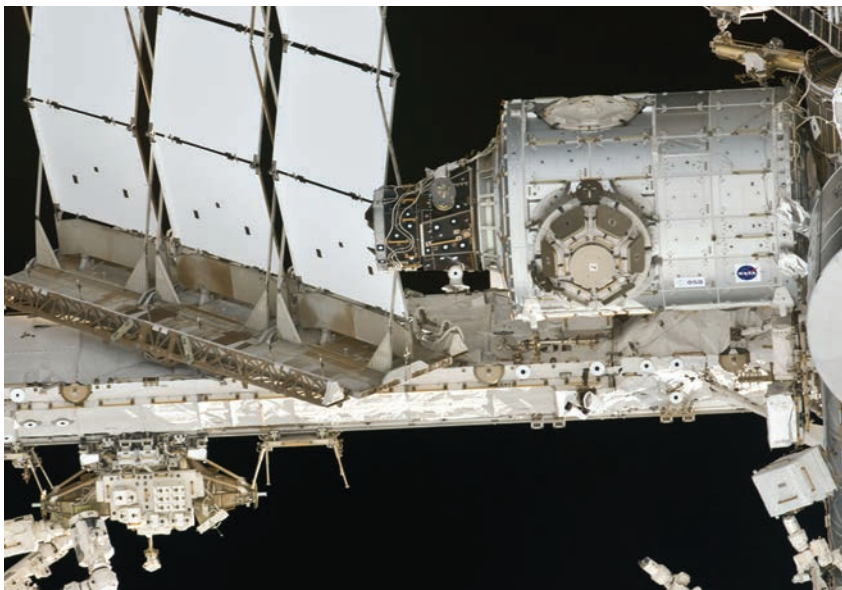
Exterior view of the P1 truss segment, Node 3/Tranquility and Cupola.
