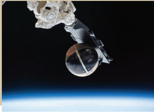
Cyclops enables the space-based launch of a new class of satellites, which are larger than cubesats but not large enough to require their own Earth-based launch vehicles.
