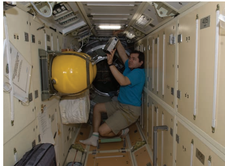
Russian cosmonaut Oleg Skripochka uses the Russian Tekh-38 VETEROK ("Breeze") science hardware to take aero-ionic concentration measurements in the Rassvet Mini-Research Module 1 (MRM1).
