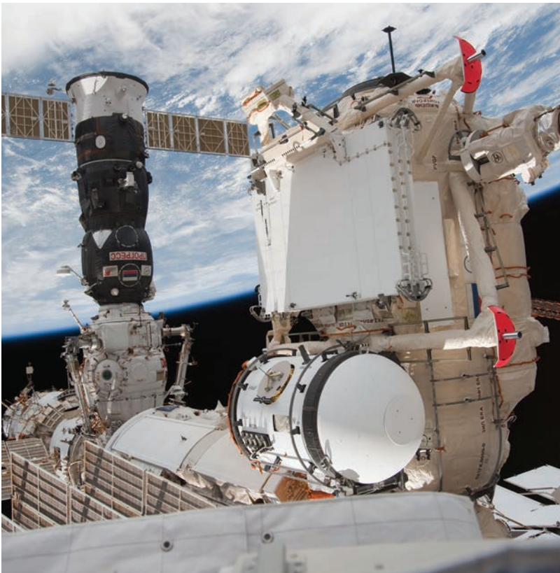
View of the Rassvet Mini-Research Module 1 (MRM1) as it is mated with the Zarya Functional Cargo Block (FCB) nadir docking port.
