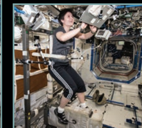
ESA astronaut Samantha Cristoforetti exercises on the Cycle Ergometer with Vibration Isolation and Stabilization (CEVIS) in the Destiny Laboratory.
