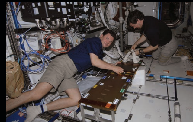
Russian cosmonaut Roman Romanenko and NASA astronaut Michael Barratt perform a detailed checkout and inspection of the HMS CMRS (Health Maintenance System/Crew Medical Restraint System) in the U.S. Lab. The boardlike CMRS allows strapping down a patient on the board with a harness for medical attention by the CMO who is also provided with restraints around the device.
