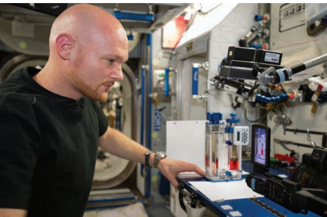
ESA astronaut Alexander Gerst conducts a session with the Capillary Flow Experiment (CFE-2) in the Harmony Node 2.
