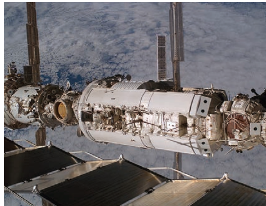
View of the FGB on orbit flanked by the Service Module and PMA-1.
