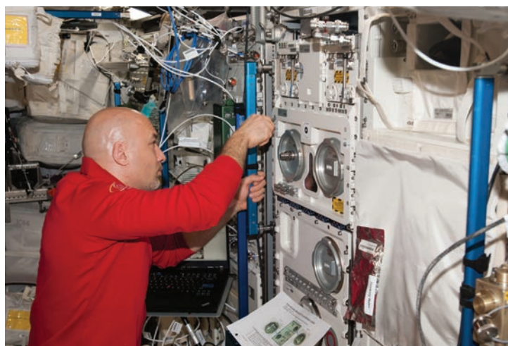
ESA astronaut Luca Parmitano works with the Biolab in the Columbus laboratory of the International Space Station. Biolab is used to perform space biology experiments on microorganisms, cells, tissue cultures, plants and small invertebrates.
