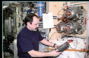
Vozdukh absorbs carbon dioxide from crew.
