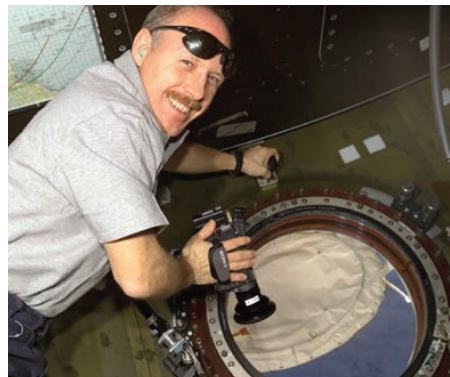
U.S. Lab in orbit, above, NASA astronaut Ken Bowersox uses camera at window with partially deployed shutter; to right, window shutter fully deployed; outer debris shields are visible.
