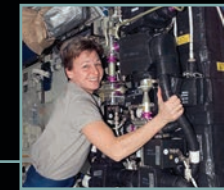
Carbon Dioxide Removal Assembly (CDRA) adsorbs carbon dioxide from crew.
