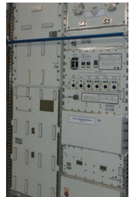
Science experiment rack accommodating a gradient heating furnace for material studies.
