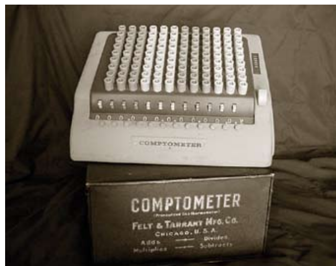
Comptometer, a mechanical calculator.
