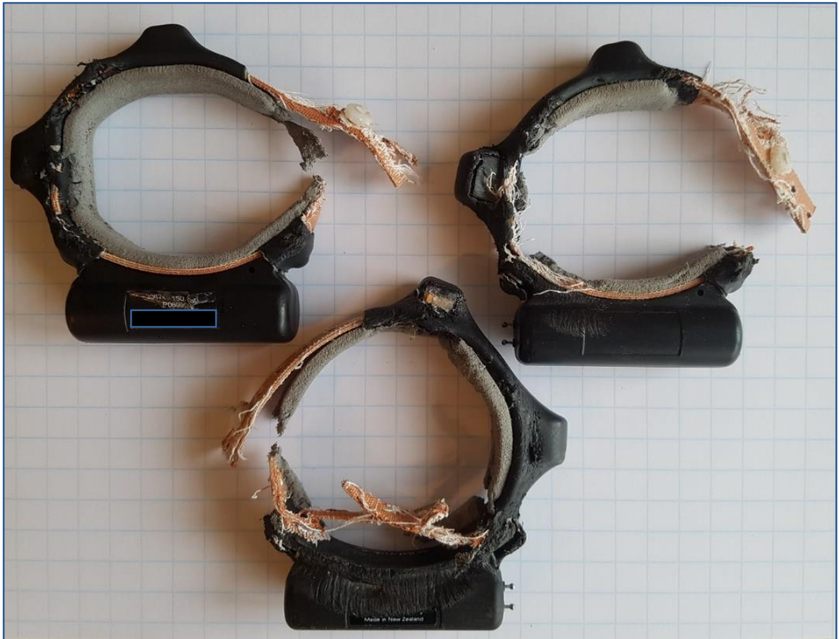
Figure 6 Examples of three Litetrack RF60 collars (LOTEK Ltd.) where coursed translocated hares slashed through the strap with their hind nails with evidence of gnawing the payload barrel. There was no evidence of predation or other extrinsic sources of mortality.
