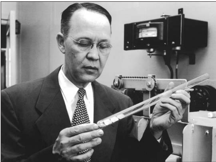
Fuller places arsenic-laced silicon into a quartz-tube furnace where he introduced a controlled amount of boron to the material, resulting in the first solar cell that could generate significant amounts of electricity.
