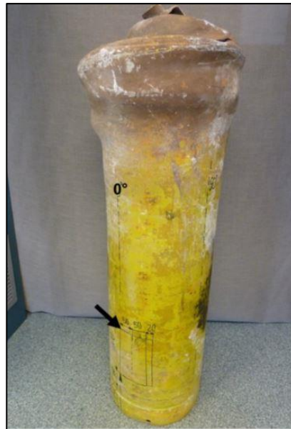
FIGURE A8.2: STEEL CUTS USED FOR THE TENSILE TEST
