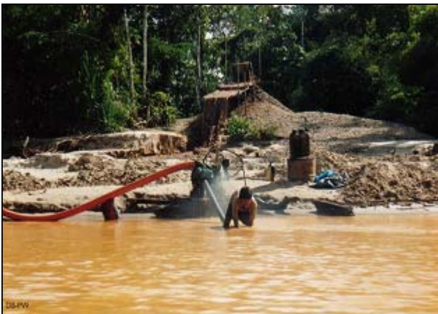
Semi-mechanized mining in Puquiri River
