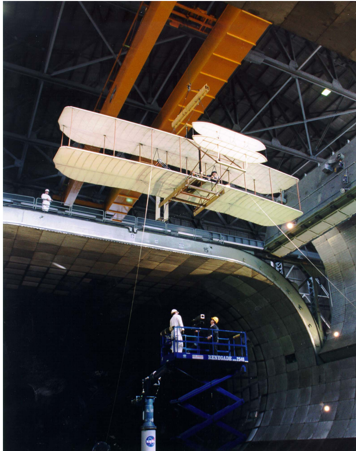
Figure 2.8: A Wright Flyer replica by the American Institute of Aeronautics and Astronautics (AIAA) undergoing testing in a NASA wind tunnel.
