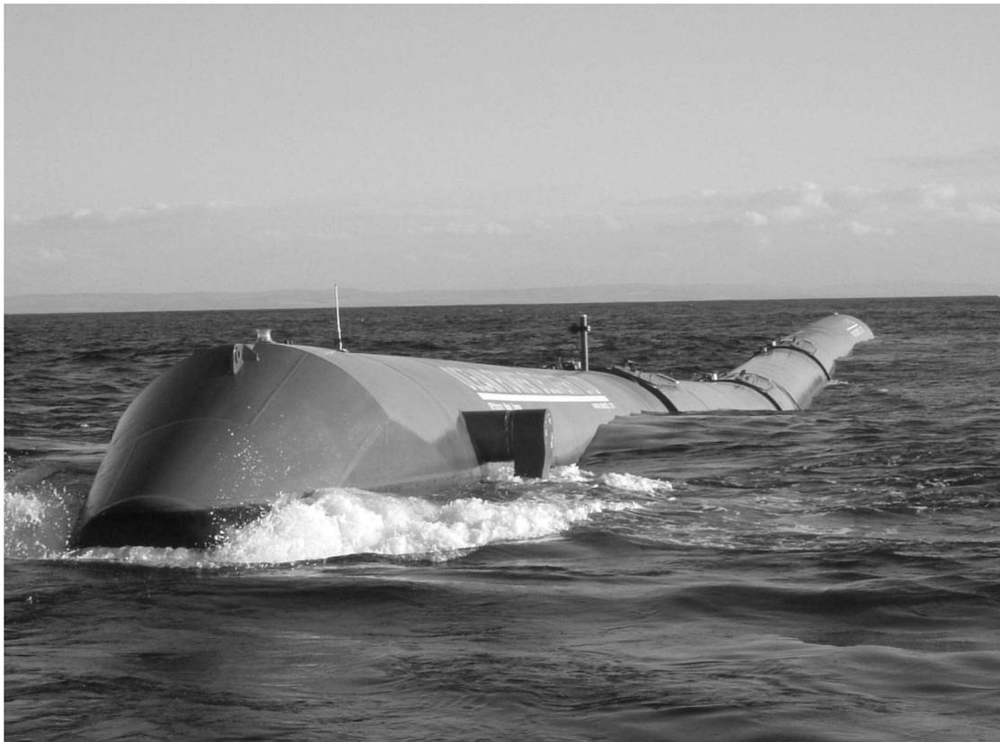
Figure 2 – Pelamis wave energy converter
