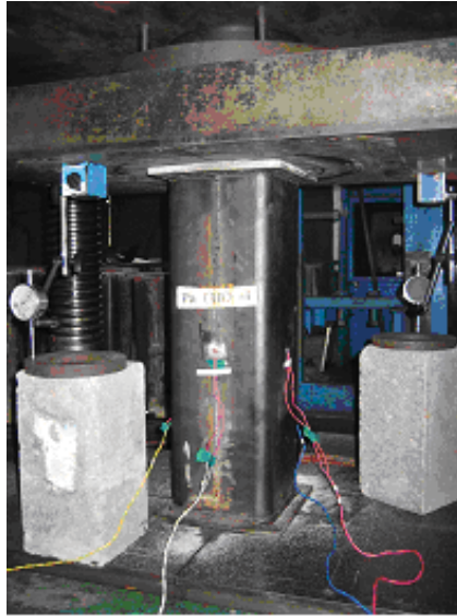
Fig. 4. Test setup of CFST-composite column specimen
