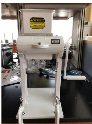
Supplemental Figure 1. Meat grinder used for simulated mastication of grapes (Weston Heavy Duty Meat Cube Tenderizer, Southern Pines, NC, USA). Images illustrate outcomes of whole grapes processed by human mastication (A) and that derived from simulated mastication (B) of red seeded table grapes.
