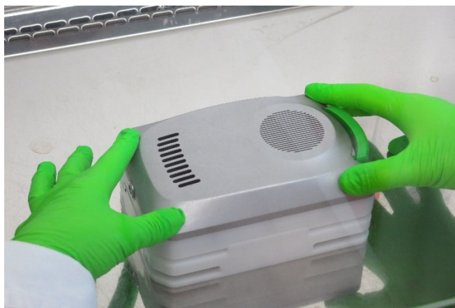
Fig. S2 Pictures of the assembling process of the OrganoTEER. A sterile electrode board (a) is inserted into an OrganoPlate (b) using a guiding plate holder (c) . The measurement unit is then connected on top of the electrode board (d) .
