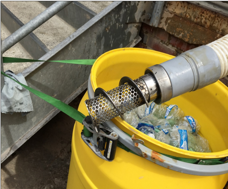
Figure 3. A Deflecting Head where the auger and screen rotate together.
