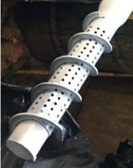
Figure 4. A Clearing Head prototype. Under a clearing mechanism, the screen can either rotate about a stationary auger or an auger can rotate about a stationary screen.
