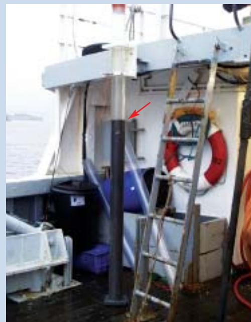
Fig. 9. Sediment core recovered from Loch Etive using the new design spear corer. The intact sediment-water interface is indicated by the arrow. © Tracy Shimmield
