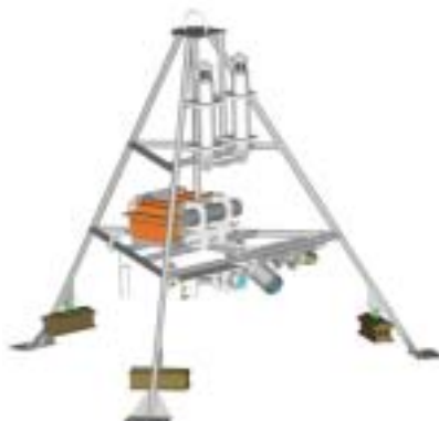
Fig. 26. Deep-sea benthic group's Photo Lander. At the end of its mission, which may last from days to weeks, the lander is commanded to release the ballast suspended from each of its three legs and a buoyant sphere (not shown) returns it to the surface where it is retrieved by the research ship. On-board time-lapse cameras record activity on the seabed while a current meter and optical instruments record the near seabed water flow and the particles suspended in it.
