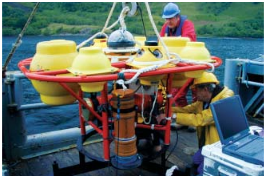
Fig. 43. The prototype HOMER profiler system is prepared for deployment to the bottom of Loch Etive. The buoyant central glass sphere, containing an electronics package and a number of sensors, is repeatedly released and retrieved by a winch in the seabed package. Data are transferred between the sphere and the seabed docking station via an infra-red link. This profiling technology is being developed at SAMS to furnish a number of research initiatives with a key new instrumentation capability.
