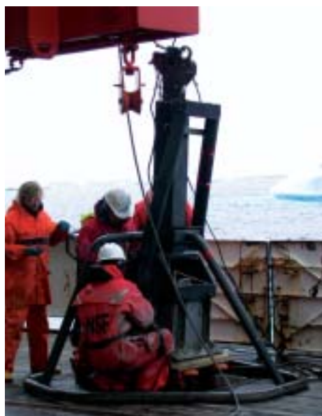
Fig. 24. Box corer with sample on board RV Polarstern among icebergs in the Weddell Sea.
