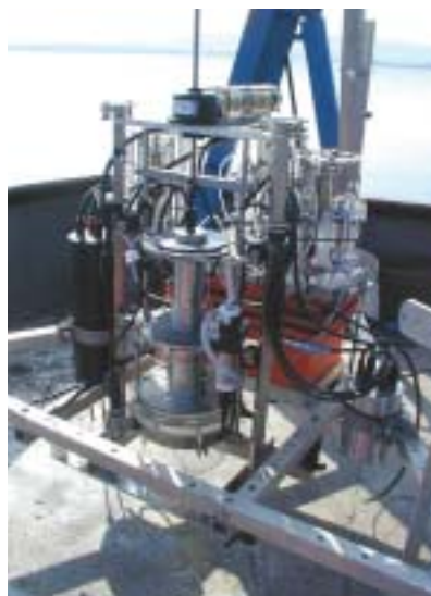
Fig. 19 (left). The deep-sea microcosm on board RV Seòl Mara . This novel chamber has been deployed in Loch Creran to measure critical erosion thresholds of sediment under fish farm cages.
