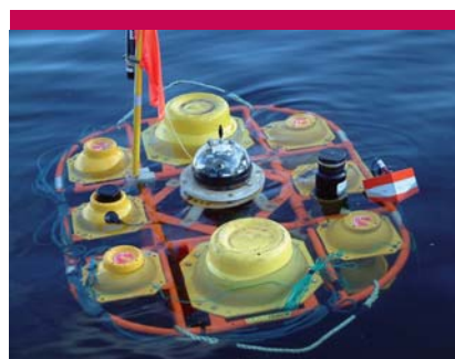
The Homer profiler being recovered after a successful trial in Loch Etive. An acoustic modem (right side of image) was used to transmit sensor data from the profiler sphere (centre of image) to a surface buoy. An Iridium satellite modem in the buoy then transmitted the data back to the laboratory. The equipment is a prototype of systems that will be deployed in remote and inhospitable locations such as the Antarctic. Photo: Luka Musić
