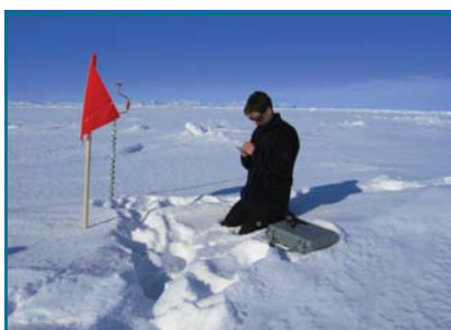
A suitcase buoy being deployed north of Svalbard.
