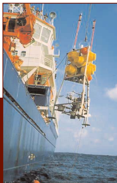
Launching the profiling lander in Sagami Bay
