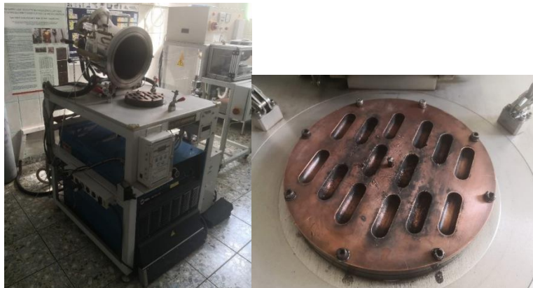
Fig.. 2.1. ABJ MRF 900 furnace and interchangeable Cu crucible
