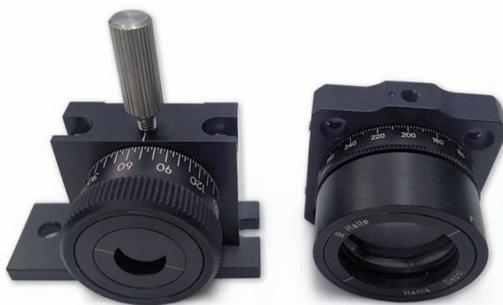
Figure 4: Polarizer (left) and depolarizer (right). The line on the polarizer mount indicates the polarization direction of the transmitted light.
