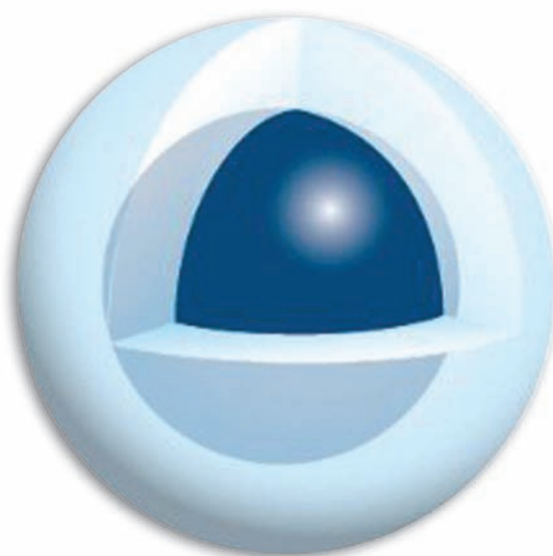
Figure 1: Schematic structure of a core shell particle with a solid core (dark blue) and the porous layer (light blue)
