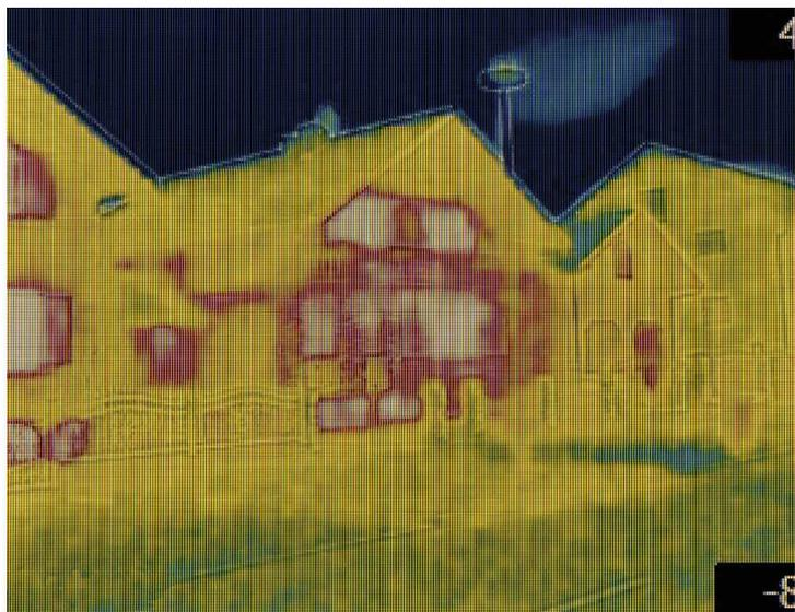
Construction thermography: surfaces with increased heat dissipation are marked in red
