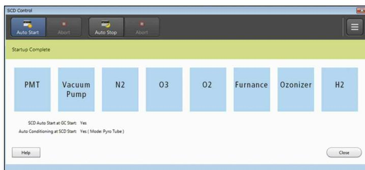
Figure 3: During automatic start-up, each module of the SCD-2030 is started up step by step. Interim intervention by the user is no longer required before readiness for measurement.
