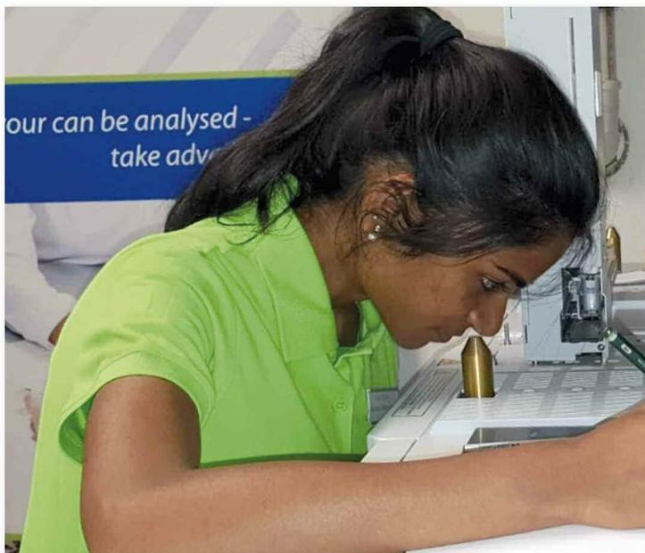
Figure 4: Sniffing at the FlavoLogic GC-O/GC-O/MS system
