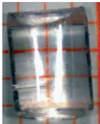
Figure 1: A typical polymer granulate in crystal clear and colorless cylindrical form on graph paper. The orange grid in the background of the granulate corresponds to 1 mm per square.
