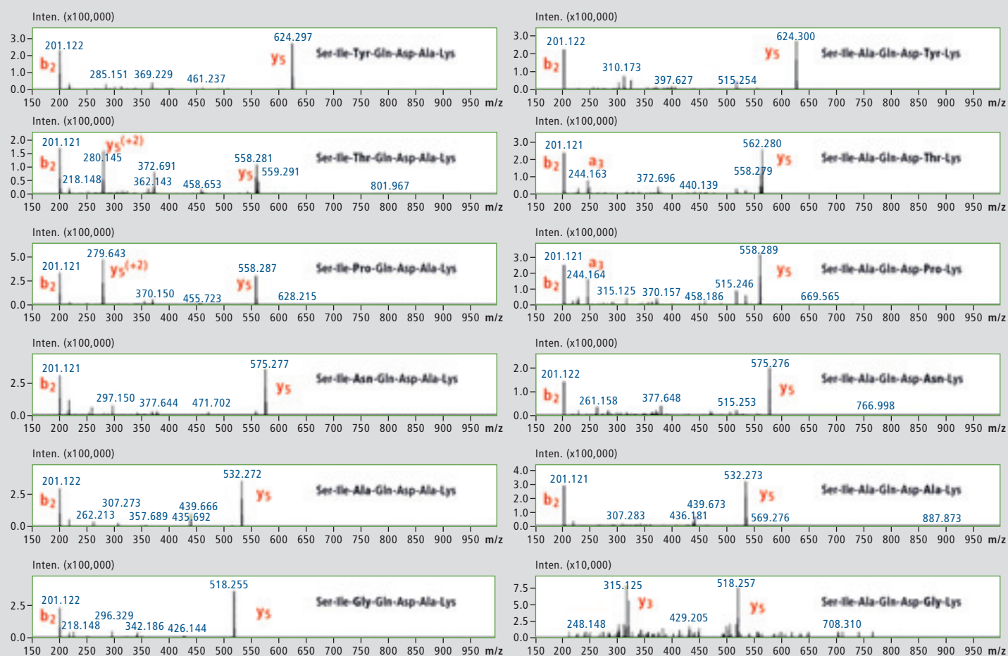
Figure 3: MS 2 analysis of peptide library subsets, [M+2H] 2+ ions were selected as precursors
