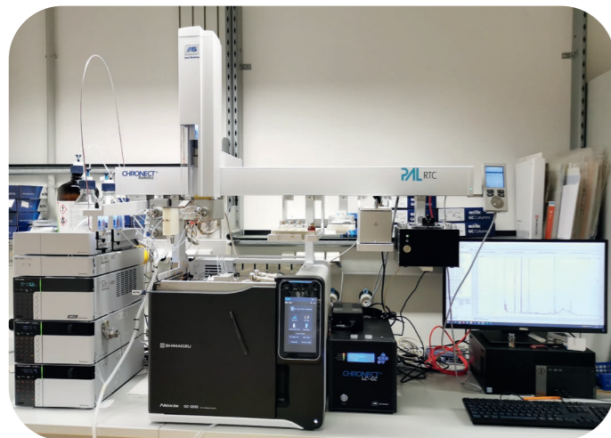
Figure 1: Online-coupled HPLC-GC-FID (left) and chromatogram of typical mineral oil (right, black = MOSH, pink = MOAH)
