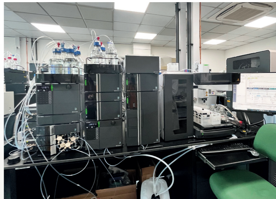
Figure 3: One of the two Shimadzu UFPLC systems in the lab of the Preparative and Isolation Chemistry Team at Syngenta. The system uses trapping cartridges to collect fractions, each of which can hold ca. 100 mg of material, and can be flushed to change solvent, pH, remove buffers – or in the case of the acid isomers – backflushed with solvent to elute the target material. The team uses a second UV detector during this backflushing step to minimize the eluent volume, which was kept to just 5 mL in this case.
