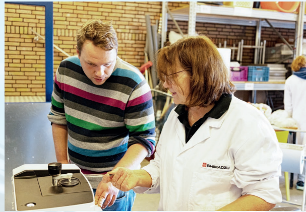
Figure 3: Workshop atmosphere during the analysis of plastic from fulmar stomachs with the Shimadzu IRSpirit infrared spectrometer
