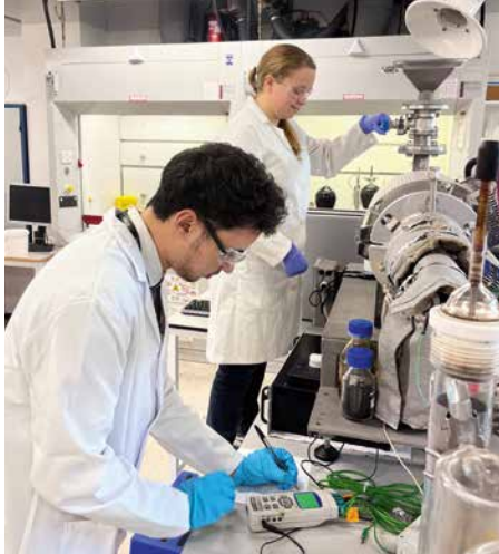
Figure 1: Adam Elaradi (Undergraduate Researcher) and Dr. Sarah Asplin (Postdoctoral Research Associate) operate the laboratory-scale intermediate pyrolysis system at EBRI. The system can take up to 300 g/h of biomass and has a maximum processing temperature of 600 °C.
