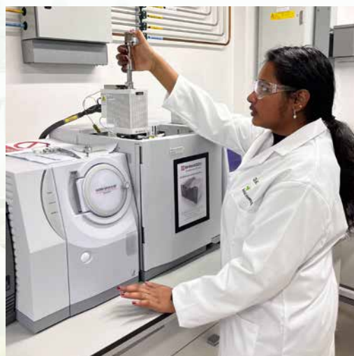
Figure 3: Anitta Xavier (Research Placement Student) injects a biomass sample into a Frontier Lab micropyrolyzer for direct transfer to the Shimadzu GCMS-QP2010 SE system
