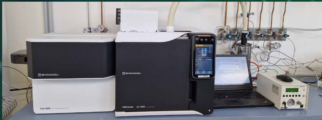
Figure 1: Nexis GC-2030 equipped with SCD-2030 detector, LVO-2030 valve box and Microjet Cryo-Trap
