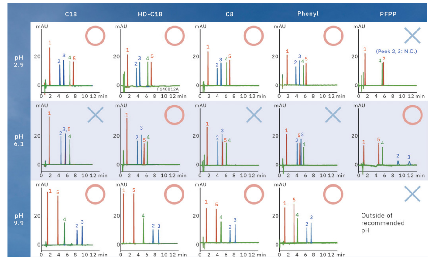
Figure 4: The Shim-pack Scepter columns offer high stability, even under low as well as high pH values. Peaks: 1: Saccharin (pKa = 2.2), 2: Dextrometorphan (pKa = 8.3), 3: Amitriptyline (pKa = 9.4), 4: n-Butylparabene (pKa = 8.3), 5: Ibuprofen (pKa = 4.4).
