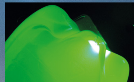
Figure 2: PET bottle bottom (caffeinated lemonade) and the fluorescence under a xenon light source. The bottle was mounted in the sample chamber of the RF-6000.
