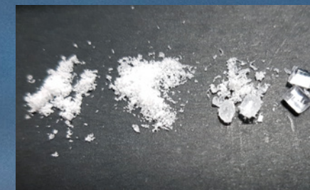
Figure 3: Screen fractions of a polycarbonate from left to right: 500-, 1,500-, 3,000- \mu\text{m} particle fractions and 5 mm granules.
