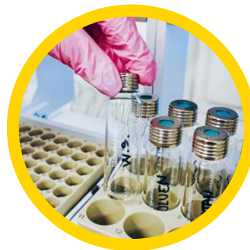
Figure 5: Multifunctional autosampler improves GCMS analysis productivity
