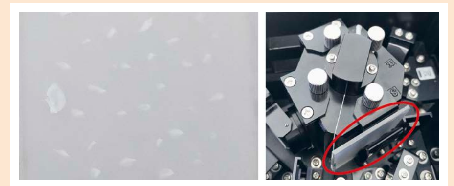
Figure 2: PMMA plate according to COLIPA before rubbing in sunscreen (left) and ready to measure, mounted at the integrating sphere (right)
