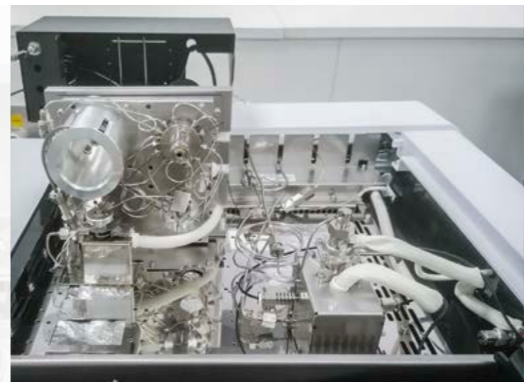
◀ ▶ Figure 3: Close-up of the custom GC valving and flowpaths in place on top of the GC. An MS detector can be added, if needed.
