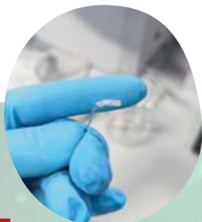
Figure 4: PDMS tube on wire
