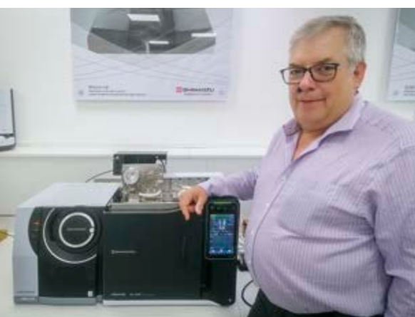
Figure 1: Custom GC expert Peter Klawitter with one of the team's bespoke instruments for the analysis of permanent gases, based on a Shimadzu GC-2030
