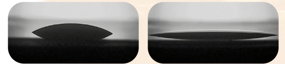
Figure 6: Light microscopic images of a PEDOT:PSS dispersion droplet on the photoactive layer P3HT:PCBM; left: without pretreatment; right: after excimer treatment
