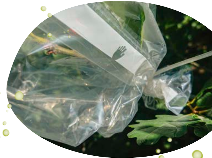
Figure 2: Oak trees wrapped in plastic oven bags to catch VOCs on PDMS
