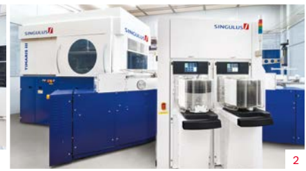
2: TIMARIS III production system for the manufacturing of 300 mm wafer
