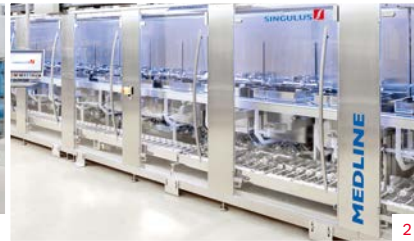
2: Large inline sputtering with vertical substrate transport
