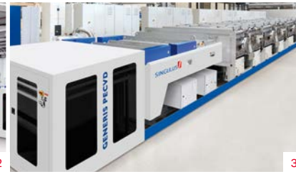
3: PECVD inline system for high-performance solar cells
