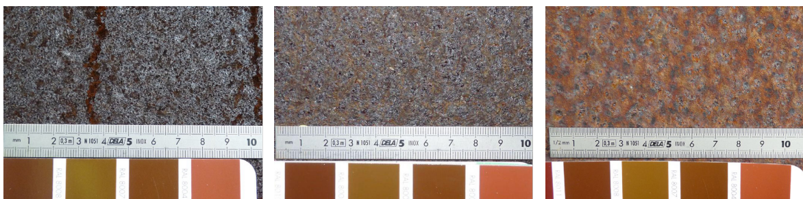
Fig. 5.2: Different appearances of the oxide layer recorded by photographs
