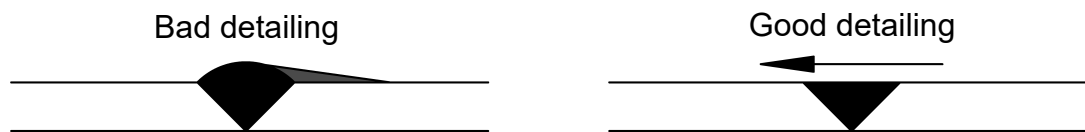
Fig. 3.5: Grinding flush of welds which otherwise form water traps
