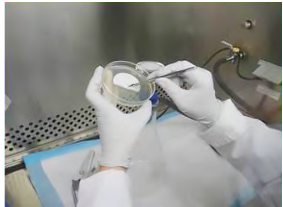
Placement of membrane filter containing microorganisms onto growth medium
