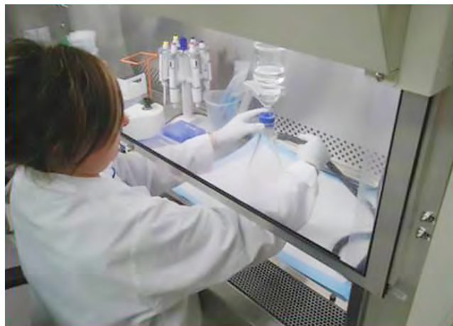
Filter collection of microorganisms present in diesel fuel
