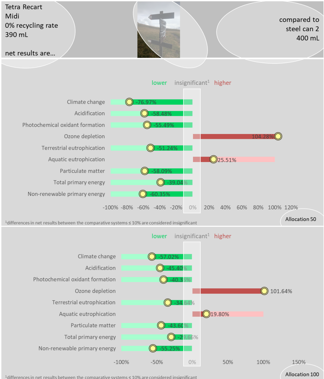
Figure 36: Comparison of net results Tetra Recart Midi 0% recycling rate and steel can 2 (400 mL) (Netherlands); allocation factor 50% and 100%
