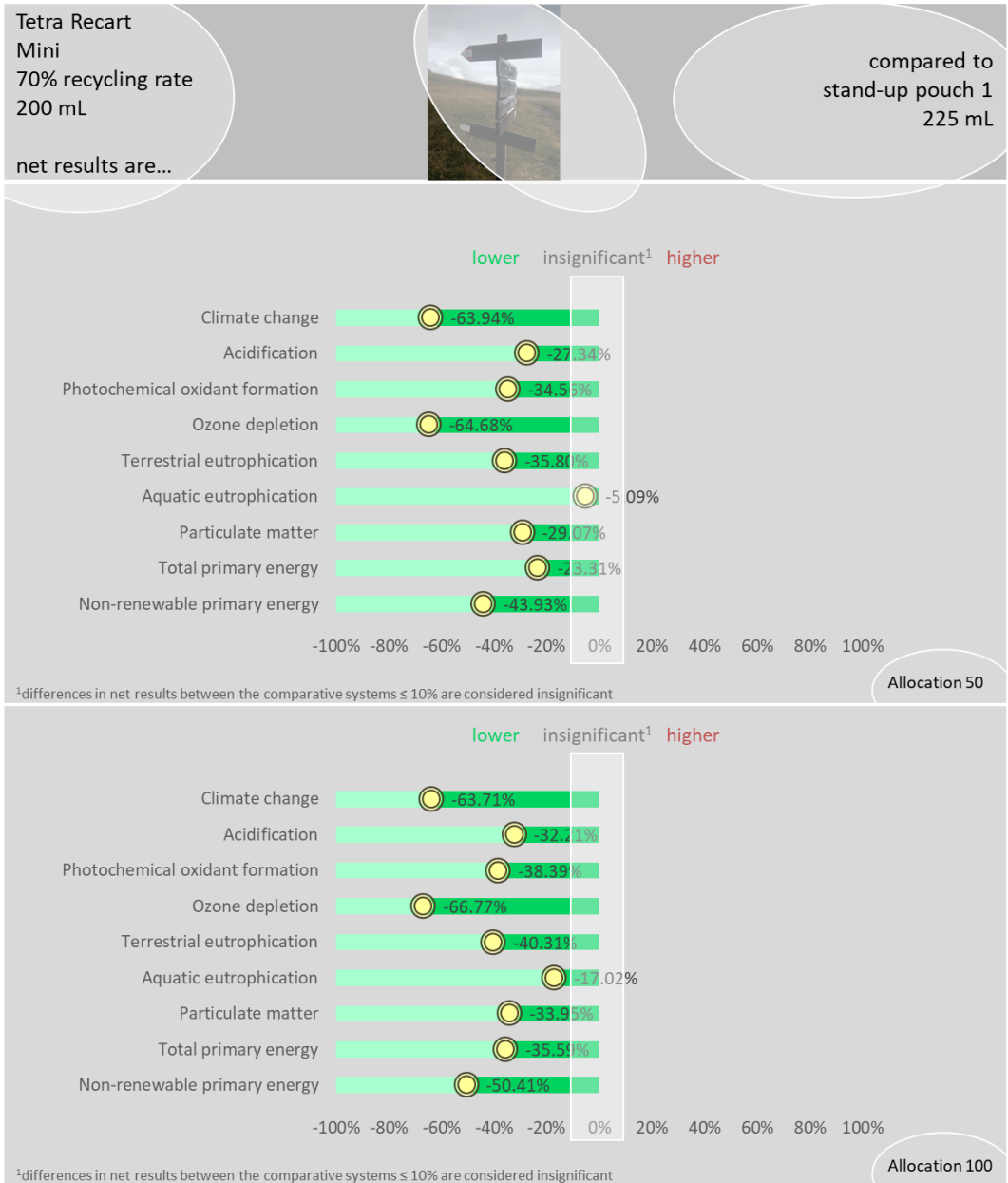
Figure 32: Comparison of net results Tetra Recart Mini 70% recycling rate and stand-up pouch 1 (225 mL) (Netherlands); allocation factor 50% and 100%
