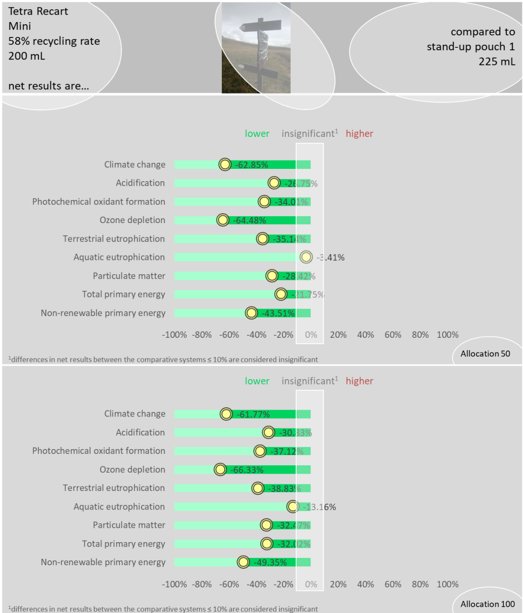
Figure 30: Comparison of net results Tetra Recart Mini 58% recycling rate and stand-up pouch 1 (225 mL) (Netherlands); allocation factor 50% and 100%
