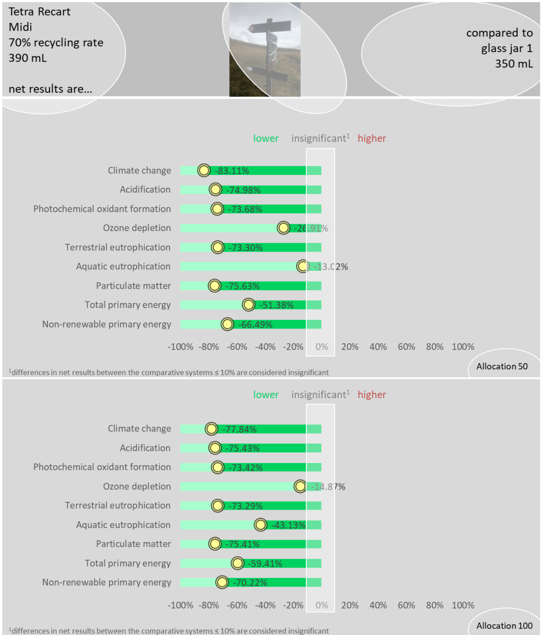
Figure 41: Comparison of net results Tetra Recart Midi 70% recycling rate and glass jar 1 (350 mL) (Netherlands); allocation factor 50% and 100%
