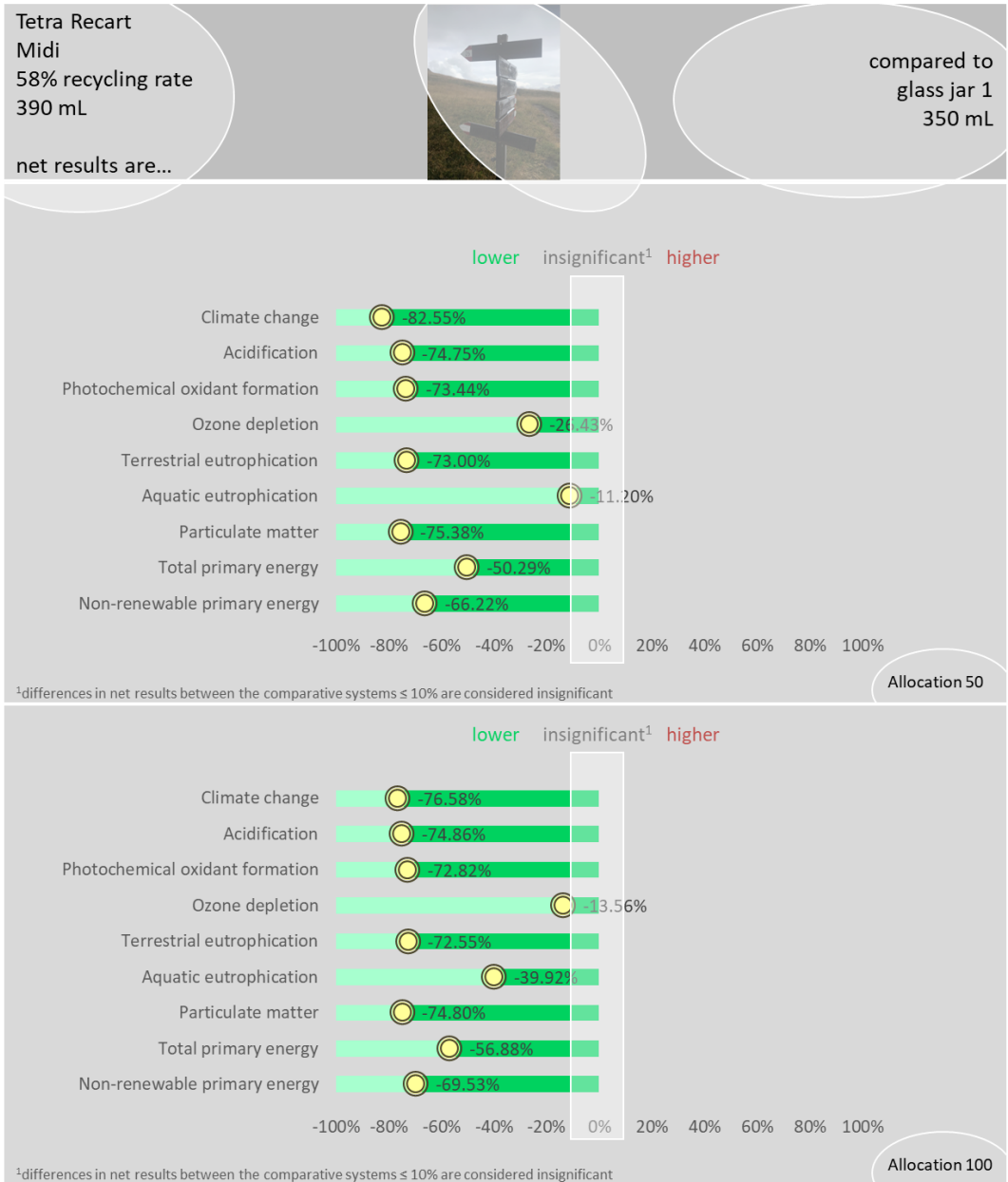
Figure 38: Comparison of net results Tetra Recart Midi 58% recycling rate and glass jar 1 (350 mL) (Netherlands); allocation factor 50% and 100%
