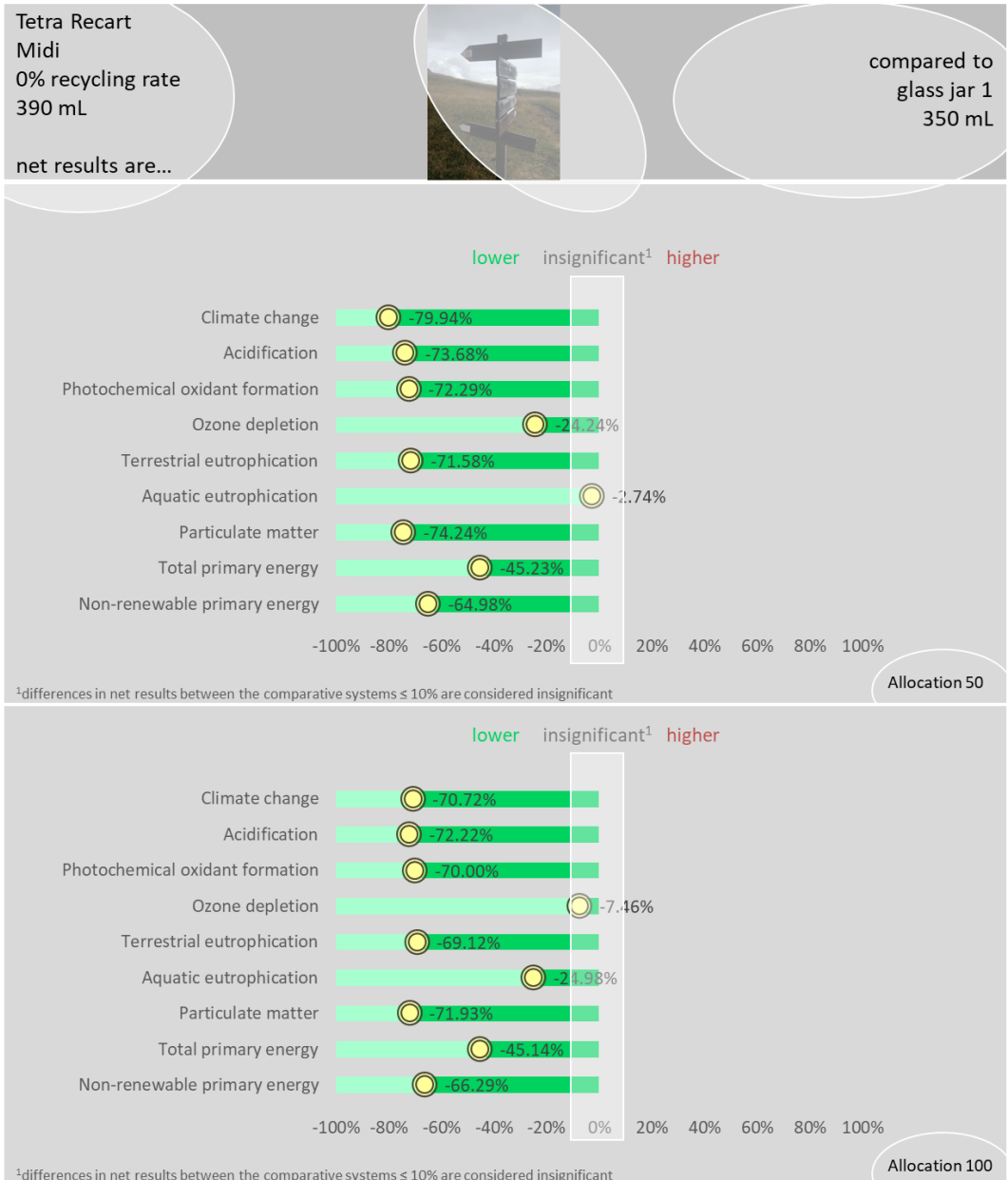
Figure 35: Comparison of net results Tetra Recart Midi 0% recycling rate and glass jar 1 (350 mL) (Netherlands); allocation factor 50% and 100%
