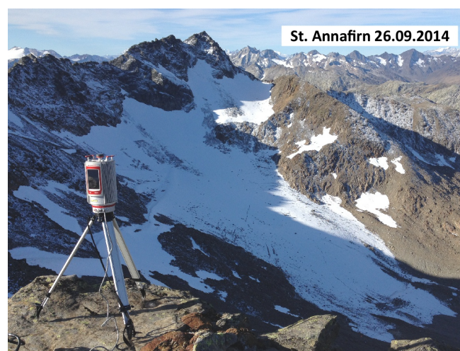
Figure 2. TLS survey of St. Annafirn in September 2014 with the Riegl VZ®-6000 terrestrial laser scanner.
