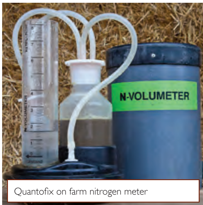
Slurry hydrometer used to estimate nutrient content of slurry
