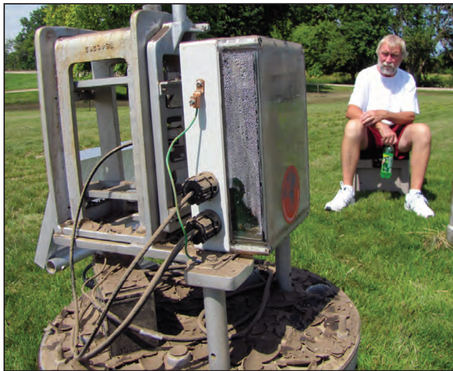
Observer Steve Gottschalk sitting next to the mud-filled Fischer-Porter recording precipitation gage.
