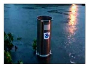
Figure 3: Rain gauge in danger of floating away
