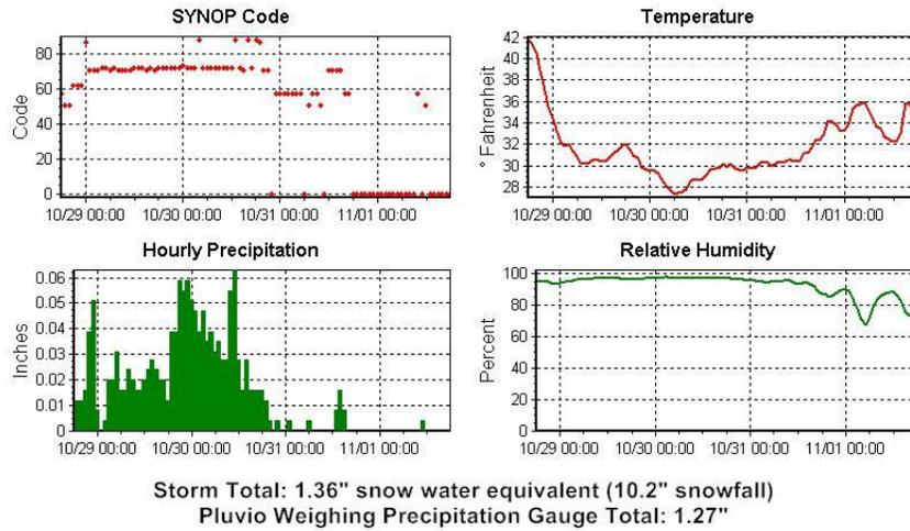
Fig. 28. Observations from Flat Springs, North Carolina (Poga Mountain). The precipitation (SYNOP) code from 71 to 73 indicates snow. Date and local standard time are on the horizontal axis of each plot. Source: Baker Perry, Ph.D., Appalachian State University.
