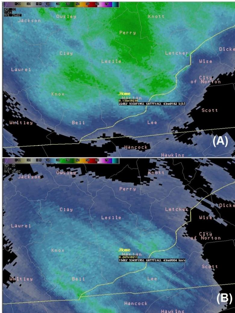
**Fig. 23.** Base reflectivity on the 1.5 degree elevation scan from (A) the KJKL radar and (B) the KMRX radar at 1159 UTC on 30 October 2012. The location marked "Home" corresponds to a point equidistant from both radars where the beam passes through.
