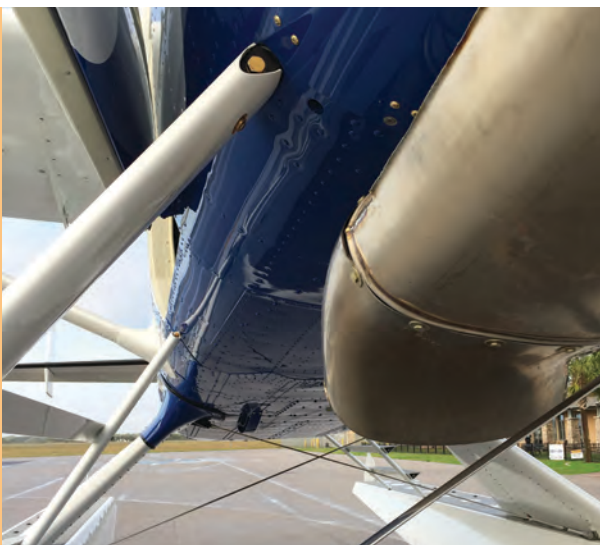
Tropic Ocean Airways' Grand Caravan EX with exhaust deflector, post-flight.
