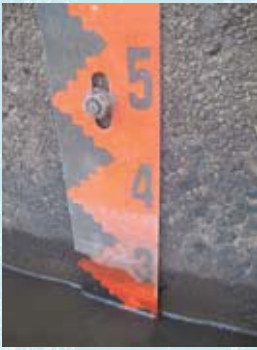
A typical gauging plate attached to a Department of Water Affairs gauging weir, where continuous records of the flow in the river are kept for use in water resource management and planning. (Photo: Cate Brown)
